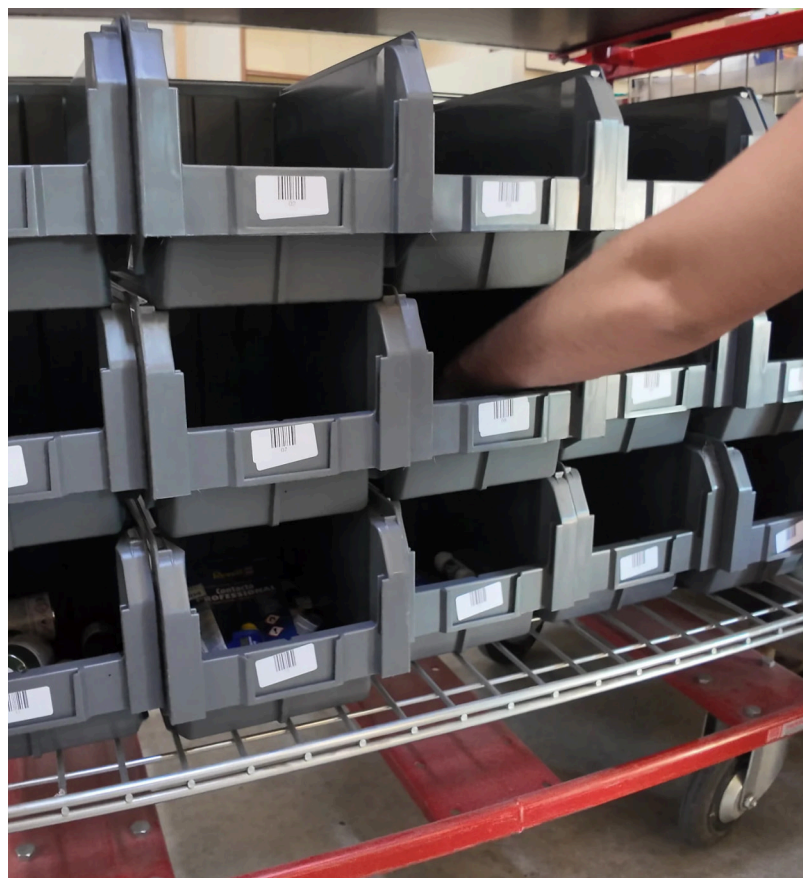
On the multi-product wave cart, one bin per order, each tagged with its own barcode.
